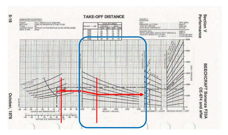
Headwind/Tailwind: The third section of the Takeoff Distance chart permits you to account for the effect of headwind or tailwind on performance. From the second reference line follow the slope of the lines in this section downward to intersect a computed headwind component, or upward to intersect a computed tailwind component on takeoff.
