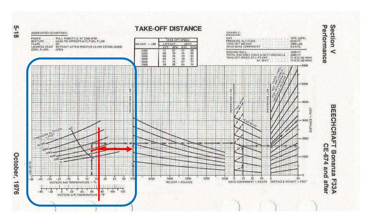
2. <u>Aircraft weight</u>. In the second section you'll adjust the calculation for the airplane's weight. From the point on the reference line you found in the first section, follow the slope of the lines in the second section downward until you intersect the airplane's weight. From that intersection, move horizontally to the next reference line, as shown below with a sample 3150-pound airplane weight:
