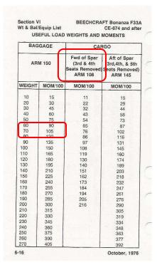
Next, account for the baggage you have on board the airplane. Let's say each of the four aboard our sample airplane has 15 pounds of baggage, all of which is secured in the aft baggage compartment. Additionally, there is 10 pounds of aircraft gear in the aft baggage area, and the pilot has a flight bag that weighs seven pounds and is kept behind the front passenger seat, at the feet of the person in the rear, right seat.
